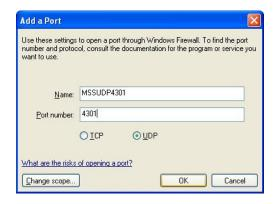
Type in the name, port number, select the appropriate radio knob, and click OK. The MSS II software uses UDP ports 4301 or 4302
